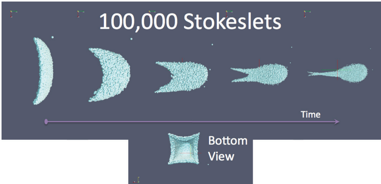
Figure 3: Simulation of 100,000 bubbles each modelled as a rigid sphere. The conduit size is much bigger than the dimensions of the modelled configuration, therefore the model is laterally unbounded. The bubbles collectively join attracted by the presence of their neighbours. It is striking how almost all bubbles merge into the collective dynamics, even when each one has a different size and therefore different buoyancy. The flow induced in the surrounding magma is the main driver of their dynamics. This model illustrates how a big sets of separate bubbles is able to collectively rise and coalesce into a larger bubble.
