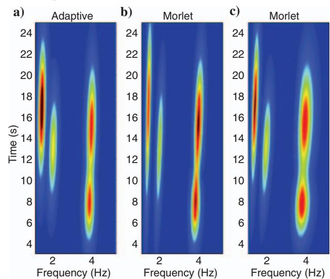
Figure 9. Results of (a) the adaptive-wavelet analysis and (b, c) the Morlet-wavelet analysis for the signal in Figure 8. Different scaling parameters were used for the Morlet wavelets to achieve the best frequency or time representations in (b) and (c).
