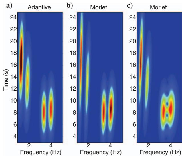
Figure 7. Time-frequency amplitude representation of the synthetic wave packet portrayed in Figure 6. (a) Results from the adaptive-wavelet analysis are presented in comparison with (b) and (c) results from the Morlet-wavelet analysis, where different scaling parameters were used to achieve the best frequency or time representations.
