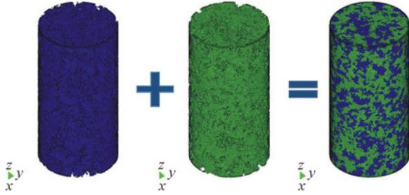
**Figure 1.** The randomly distributed spatial granularity specimen consisted of ice and rock. It displays our finite element numerical model created by randomly mixed ice and rock. The left figure shows the ice and rock's spatial distribution, and each color represents one kind of component. The right figure shows the randomly distributed spatial configurations of ice and rock.
