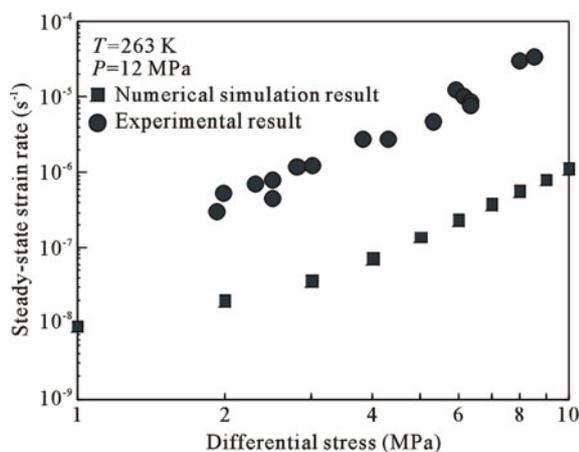
**Figure 4. Steady-state strain rate versus differential stress for comparison at a fixed ice fraction of 48% with fixed temperature and pressure. Our numerical simulation results are compared with the experimental results (Mangold, 2003).**
