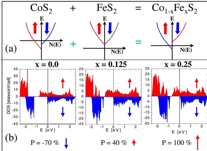
FIG. 1 (color online). (a) Schematic depiction of the basic concept of composition control of  $E_F$  and  $P$  in  $\text{Co}_{1-x}\text{Fe}_x\text{S}_2$ . (b) Calculated DOS for  $x = 0.00, 0.125,$  and  $0.25$ . The value of  $P$  in each case is shown underneath the figure.  $E_F$  is taken as the zero point of energy.
