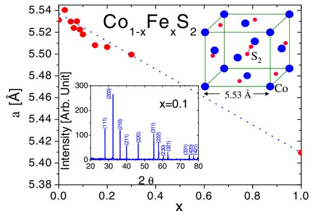
FIG. 2 (color online).  $x$  dependence of the experimental lattice parameter. Solid points are data, while the blue or dark grey dotted line is Vegard's law. Lower inset: X-ray powder diffraction from a representative sample ( $x = 0.10$ ). Upper inset: Crystal structure of  $\text{Co}_{1-x}\text{Fe}_x\text{S}_2$ . Blue or dark grey circles are the Co(Fe) atoms; red or light grey circles represent the S atoms.
