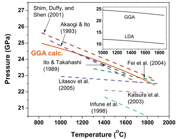
**Figure 3.** Computed postspinel transition boundary compared with experimental measurements. Inset compares predicted GGA and LDA phase boundaries. At 1900 K the Clapeyron slopes are in MPa/K: GGA,  $-2.9$ ; LDA,  $-2.6$ ; Ito and Takahashi [1989],  $-2.8$ ; Akaogi and Ito [1993],  $-3.0$ ; Irifune *et al.* [1998],  $\sim -2.5$ ; Shim *et al.* [2001],  $-2.75$ ; Katsura *et al.* [2003],  $\sim -2 - -0.4$ ; Fei *et al.* [2004],  $-1.3$ ; Litasov *et al.* [2005],  $-0.5$ .
